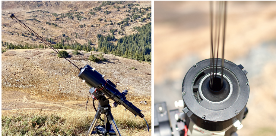
Figure 1. Overview of CATEcor coronagraph assembly and CATE telescope setup during field tests on Loveland Pass in Colorado (left). CATEcor assembly aperture in the coronagraph occulter umbra during the same field test (right).
