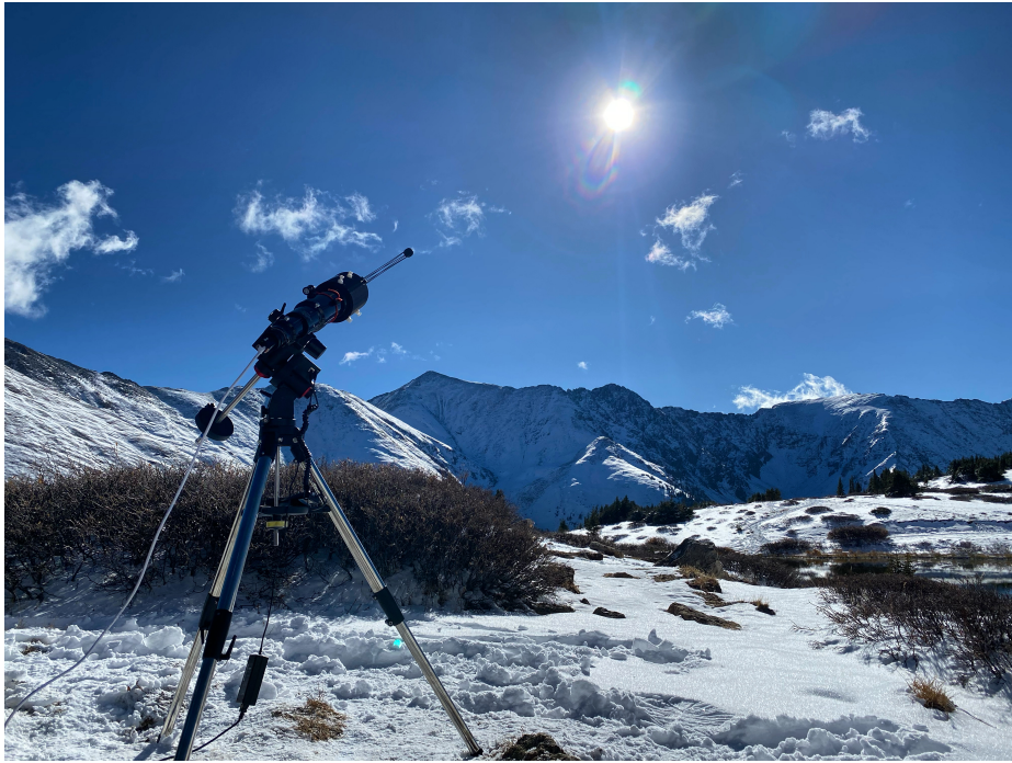
Figure 3. The CATEcor telescope and coronagraph assembly at Pass Lake, just below Loveland Pass, in Colorado, during the early phases of the 14 October 2023 partial eclipse. Our observing site offered completely unobstructed views to the south, over the Arapaho Basin Ski Area. A snowstorm on 12 October complicated working conditions at the site, but helped to suppress airborne dust.
